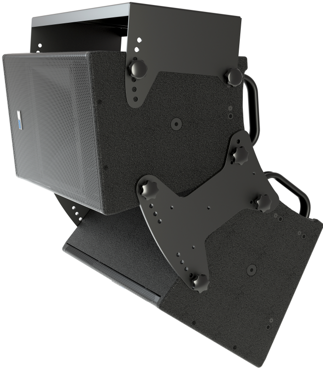
Figure 7: MTB-X40 Suspending two ULTRA-X40 Vertically Using Two MCP50-x40 Cluster Plates
