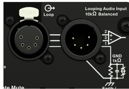
Figure 18: XLR 5-Pin Audio Connectors, Input and Loop Output
